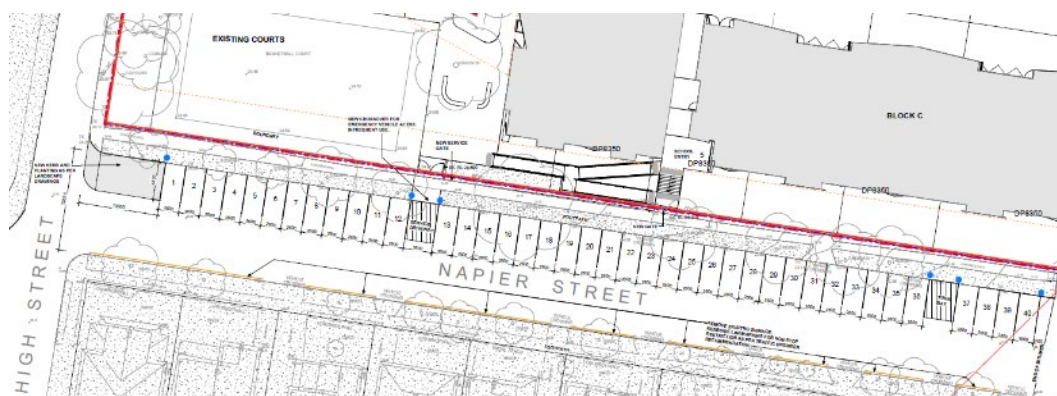
Figure 18 Proposed Realigned Parking on Napier Street
